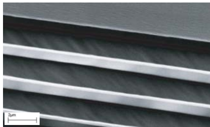
Figure C.3: SiNWs etched in a Si (110) wafer. Etch stops on vertical {111} planes.
