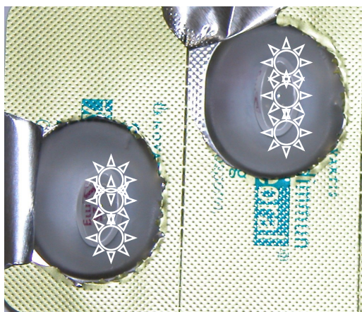
Figure 20: The three measuring spots in the 25mg blister cup.
