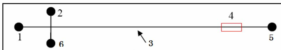
Figure 4. Scheme of a microchip, 1: electrolyte inlet, 2: sample inlet, 3: separation channel, 4: detector, 5: electrolyte outlet, 6: sample outlet
