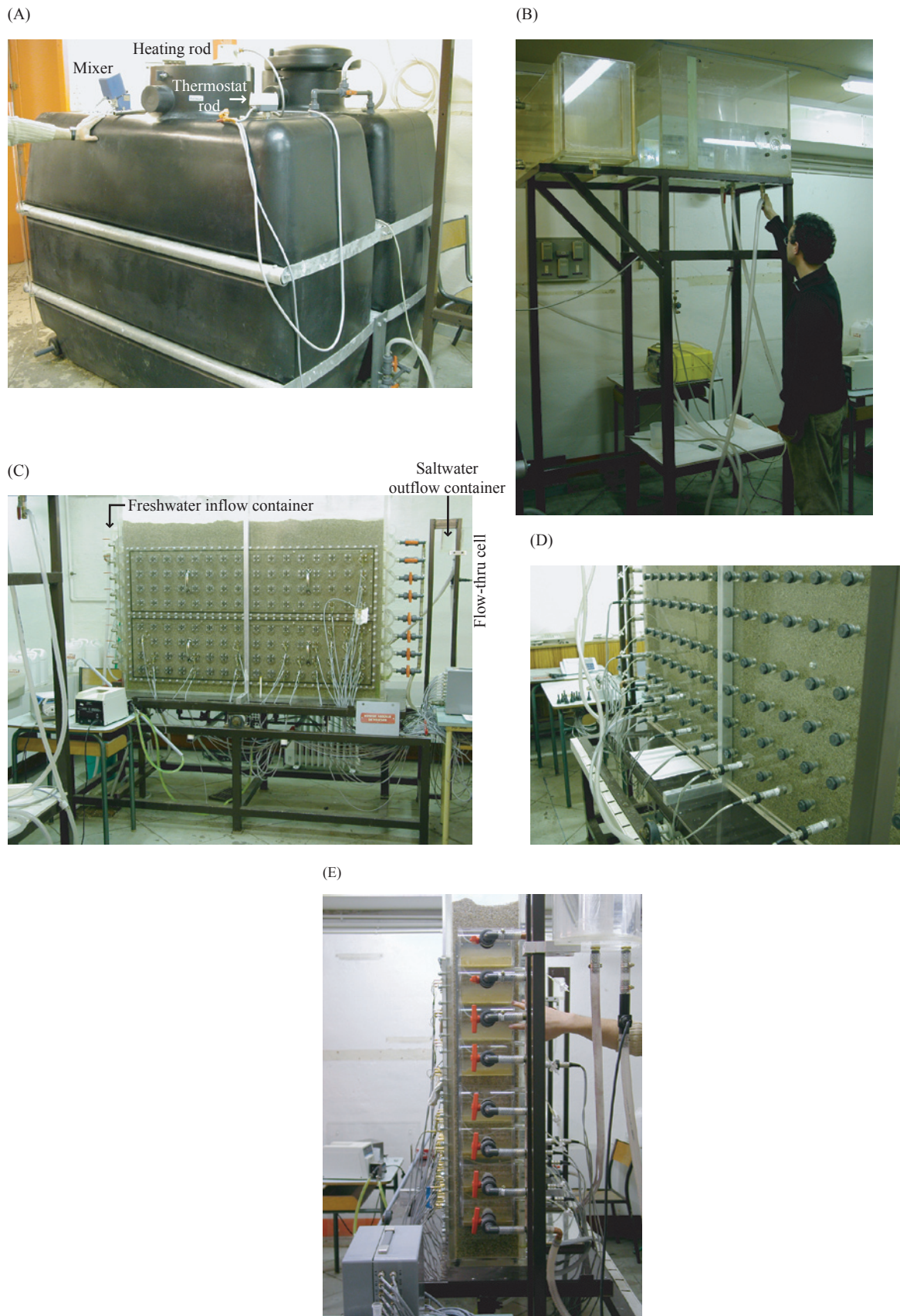
Figure 6.3 Photographs of the (A) two freshwater reservoirs with heating rod, thermostat rod and mixer; the (B) intermediate freshwater reservoir; the (C) front view of the 2D flow tank during an experiment; the (D) back view of the 2D flow tank with pressure transmitters; and (E) view of the outflow end.
