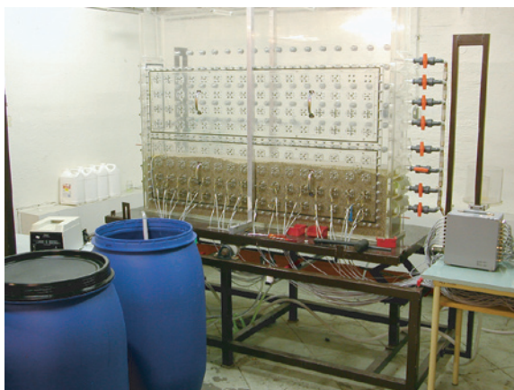
Figure 5.4 Experimental setup for tests in the (A) 2D flow tank and in the (B) small container, respectively. The horizontal saltwater layer can be clearly observed in (B) (reddish color of the brine, yellowish color of the transition zone).
