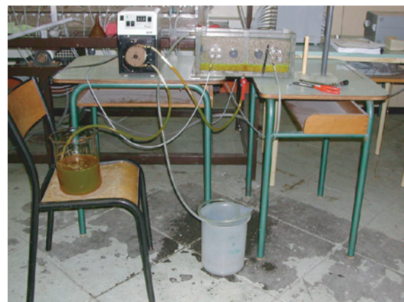
Figure 5.4 Experimental setup for tests in the (A) 2D flow tank and in the (B) small container, respectively. The horizontal saltwater layer can be clearly observed in (B) (reddish color of the brine, yellowish color of the transition zone).
