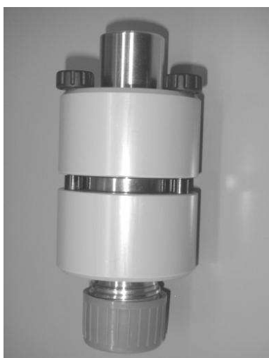
Figure 21: Example of the assembled metal mixing element before inserting in the Turbula ® .
