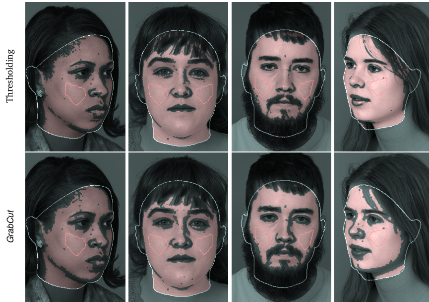
Figure 4.14: More segmentation results comparing the thresholding and the GrabCut method, both applied on the texture similarity output E_{ts}^k(R^-(I)) . The image samples were chosen with focus on the problem of segmenting out different kinds of hair.
