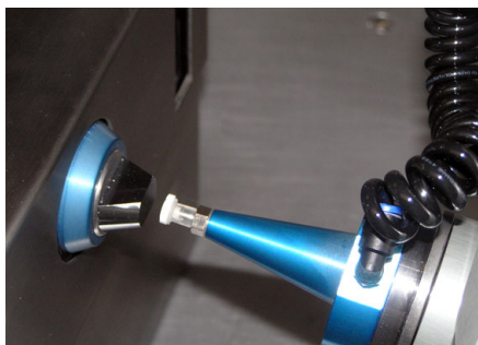
Figure 3.11 Close-up of tablet on robot arm during terahertz analysis with TPI imaga 2000 system (picture: TeraView Ltd, Cambridge, UK).
