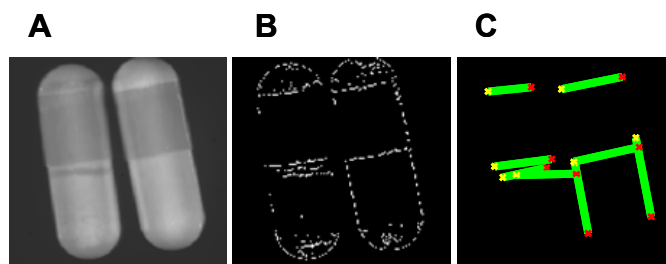
Figure 2.15 A: image of capsules at 1870 nm, left capsule has a briquette with a crack, right capsule contains uncompressed granules. B: Sobel edge detection of image A, contours and crack of the capsules are detected. C: Hough line detection of image B, some of the contours are detected as well as the crack.
