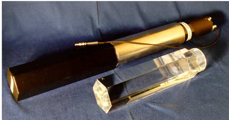
Figure 2.5: Picture of a single BaF_2 crystal and a fully mounted detector element with its photomultiplier where the crystal is covered with black tape.
