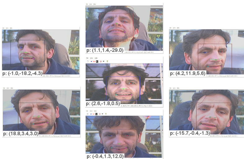
Figure 4-4: Pose Estimation integrated in FaFaFeDe For visualisation purposes, we integrated the pose estimation to the FaFaFeDe live application. The three angles p : ( \langle roll \rangle , \langle yaw \rangle , \langle pitch \rangle ) are shown within the status bar of the application.
