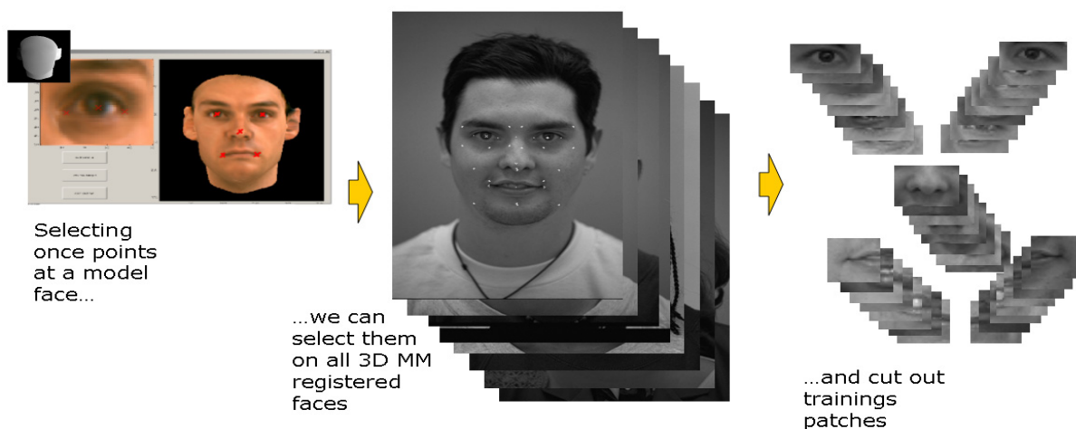
Figure 3-3: Generation of training sets from the FERET database Selecting once points at a random model face, we can select them on all 3D MM registered faces and cut out automatically training patches from large sets of images.
