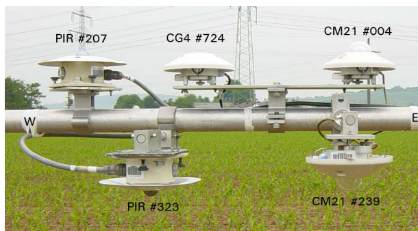
Figure 3.13: Set-up for the radiation comparison.
