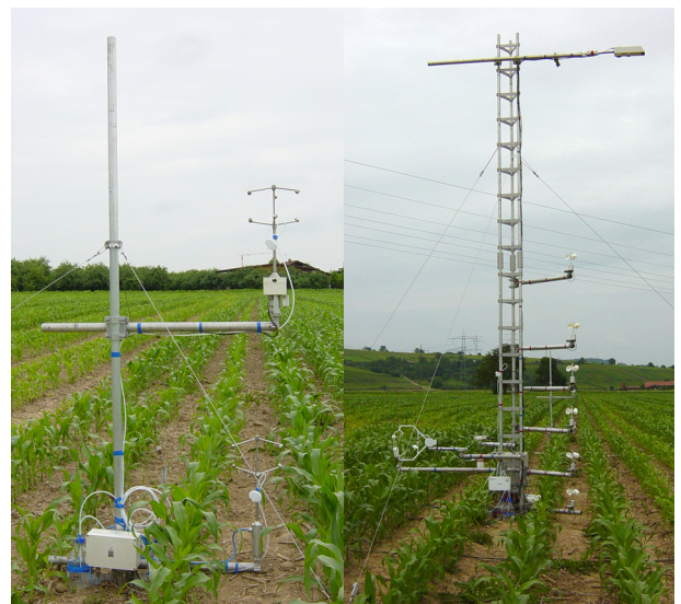
Figure 3.6: Photo of the southern advection tower on the left and the main tower with the cup profile on the right.
