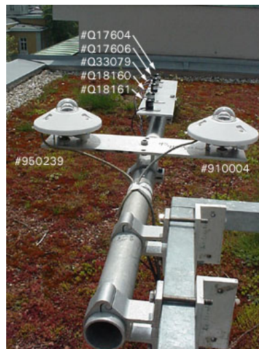
Figure 3.15: Set-up for the comparison of the PPFD sensors.
