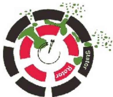
Figure 6. Functional principle of rotor-stator system
