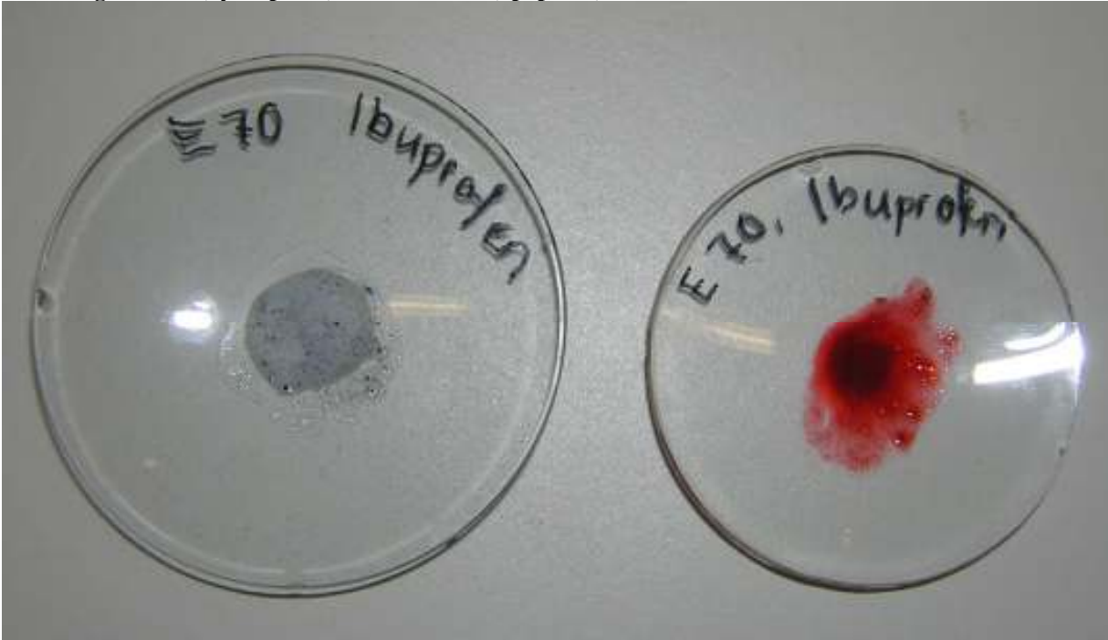
Figure 28. Dying of an emulsion comprising 70% dispersed water phase in miglyol 812N (E70) with indigocarmin (hydrophilic) and sudan III (lipophilic)
