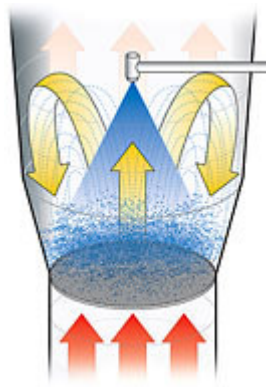
Figure 2.29: Top spray (a) and bottom spray (b) fluidized bed (Wurster) [6]
