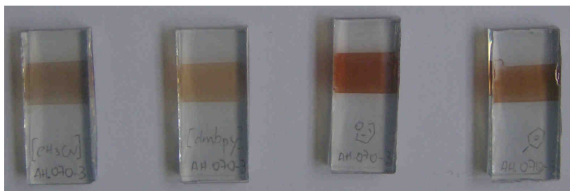
Fig. 114 TiO 2 functionalised electrodes with H 2 L6 and (from left to right) [Cu(CH 3 CN) 4 ] + , [Cu(dmbipy) 2 ] + , [Cu(L9) 2 ] + and [Cu(L1) 2 ] + .
