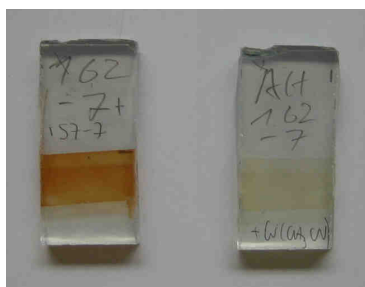
Fig. 116. TiO 2 functionalised electrodes with H 4 L24 and [Cu(L1) 2 ] + (on the left) and with H 4 L24 and [Cu(CH 3 CN) 4 ] + (on the right).
