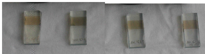
Fig. 104. Binding to \text{TiO}_2 of 1\text{mM } [\text{CuL}_2]^+ complexes with (from left to right) [\text{Cu}(\text{L18})_2][\text{PF}_6] , [\text{Cu}(\text{H}_2\text{L17})_2]\text{Cl} , [\text{Cu}(\text{L21})_2][\text{PF}_6] and [\text{Cu}(\text{H}_2\text{L22})_2]\text{Cl} . The FTO conducting glass slides were coated with 6\text{--}7\ \mu\text{m} \text{TiO}_2 nanoparticles and then immersed in solution ( \text{CH}_2\text{Cl}_2 for [\text{Cu}(\text{L18})_2][\text{PF}_6] and [\text{Cu}(\text{L21})_2][\text{PF}_6] , and DMSO for [\text{Cu}(\text{H}_2\text{L17})_2]\text{Cl} and [\text{Cu}(\text{H}_2\text{L22})_2]\text{Cl} ) for a period of 12 h.
