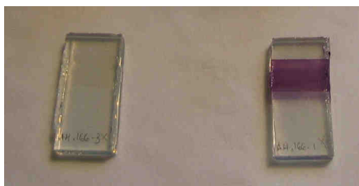
Fig. 106. Binding to \text{TiO}_2 of 1\text{mM } [\text{CuL}_2]^+ complexes in DMSO with (from left to right) [\text{Cu}(\text{H}_2\text{L26})_2][\text{PF}_6] and [\text{Cu}(\text{H}_2\text{L25})_2]\text{Cl} . The FTO conducting glass slides were coated with 6\text{-}7\ \mu\text{m} \text{TiO}_2 nanoparticles and then immersed in solution for a period of 12 h.
